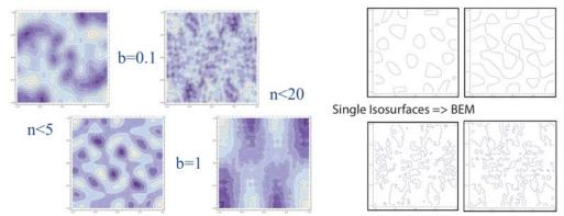
Figure 1 Synthetic porous systems generated with a Karhunen-Loeve Transform. After the extraction of single isosurfaces a BEM solution is calculated.
