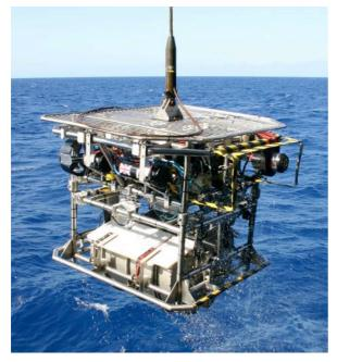
Figure 3: The *HyBIS* ROTV being deployed from the RRS *James Cook*.
