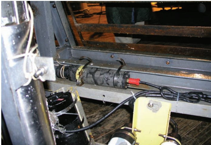
Figure 1: Deep-sea, in-situ electrochemical sensor on the hydrothermal deep-tow.
