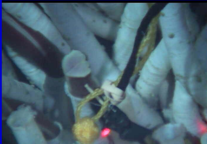
ISEA = In Situ Electrochemical Analyzer
