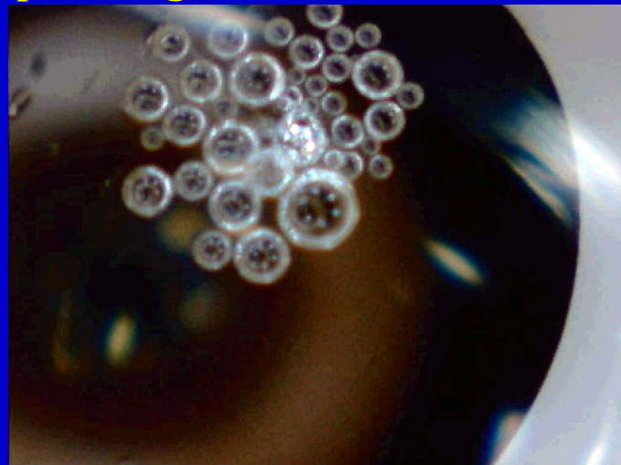
After epoxy injection before sanding and polishing - GLASS
