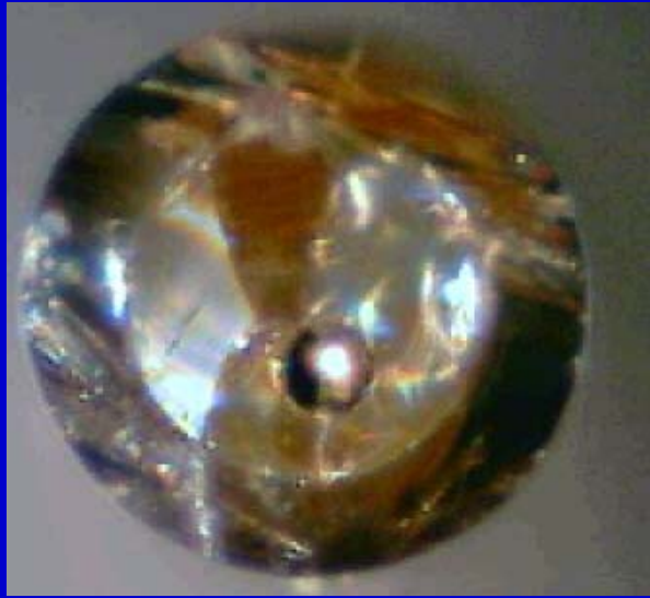
After epoxy injection before sanding and polishing - GLASS
